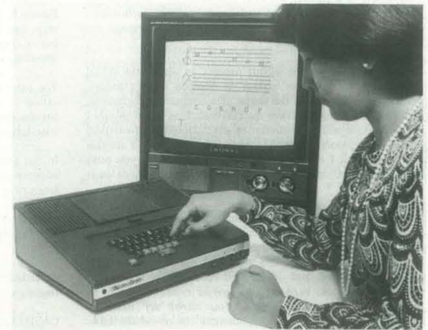
In Music Teacher I, as you type in notes they're displayed on the screen's staff and played over the TV's speaker.
